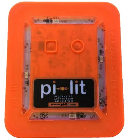
batteries. The green or red LED will flash the status of the batteries. 5 green flashes = full batteries, 4 green flashes = full batteries, 3 green flashes = good batteries, 2 red flashes = low batteries, 1 red flash = very low batteries. We suggest changing batteries between the 3 green flashes and 2 red flashes.
